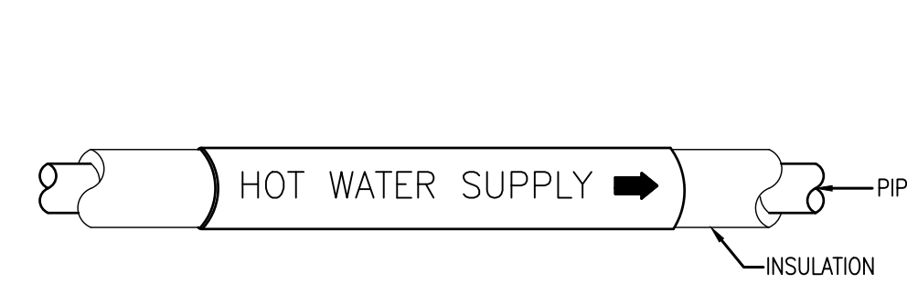
3 TYPICAL PIPE IDENTIFICATION NTS
