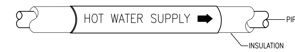
4 TYPICAL PIPE IDENTIFICATION M-601 NTS
