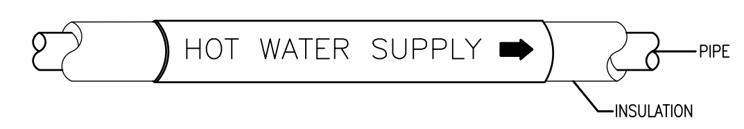
4 TYPICAL PIPE IDENTIFICATION MH501 NTS
