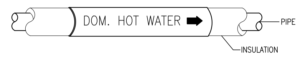
5 TYPICAL PIPE IDENTIFICATION M103 NTS
