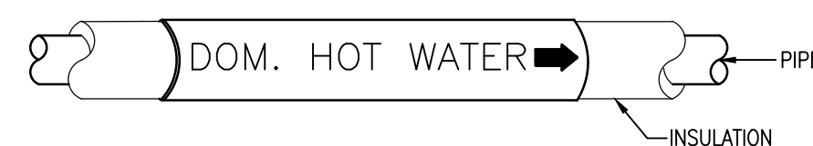
5 TYPICAL PIPE IDENTIFICATION MH501 NTS
